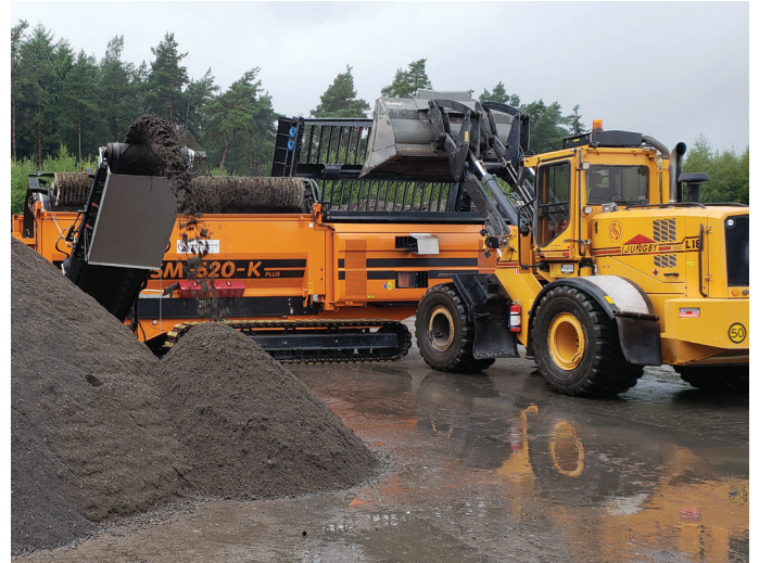
RemBind being applied to treat PFAS soil in Europe
