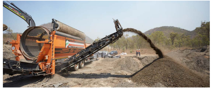
Soil Treatment Using a Mobile Trommel Screen
