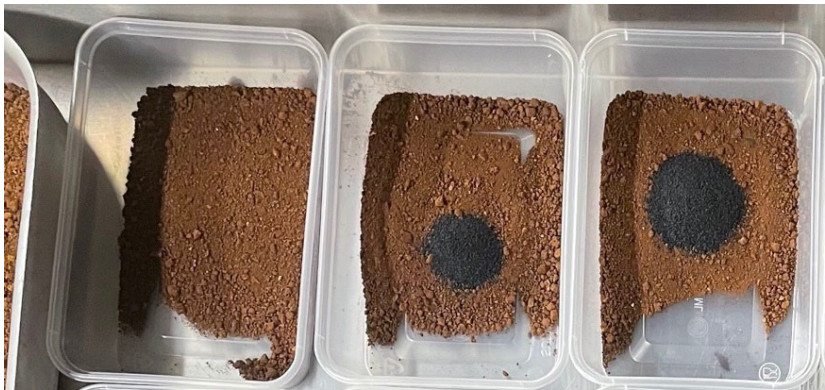
1. Screen soil, dose reagents (0% to 5%)
